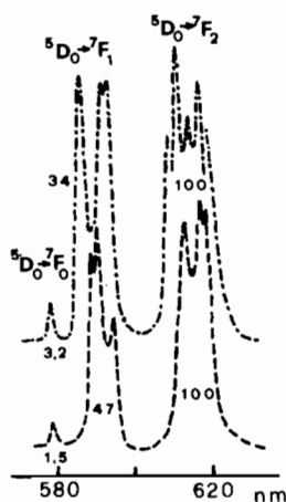
Fig. 2. Emission spectra at 77 K of: (---) \text{Eu}(4\text{-AN})_3 \cdot 3\text{H}_2\text{O} ; (-.-) \text{Eu}(4\text{-AN})_3 . Assignments and relative intensity (%) are also shown.
